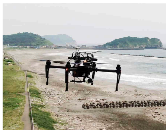
When a drone automatically recognizes people on the fly, it approaches to the people so that they can send SOS messages via the drone to the outside of a disaster area
